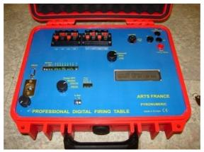
This machine functions by using the same equipment (receivers & power station) and by following the same process as the manual table. It replaces the 960 firing table and gives you much more: up to 4000 lines programmed to  $1/10^{th}$  of a second (or to  $1/20^{th}$  by using 32 sequencers), which can be transformed into 4000 x 32 = 128 000 lines set up wherever you chose by adding 32 programmed sequencers.
