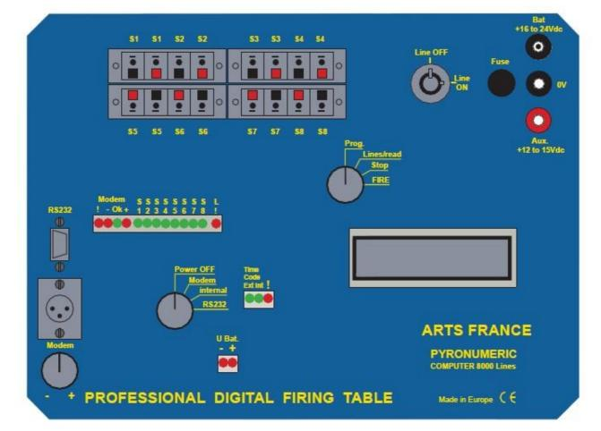
2.1 The equipment 2.1.1. Inputs COM RS232 Line 1 DB9/F outlet connected to one of the PC's COMs to program the firing sequence and store it in the firing table's memory.
