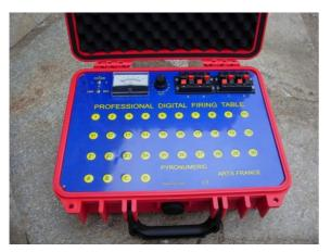
It facilitates the control of 8 "Systems", each of them connected with a couple of cords to decoding receivers and 30 relay units (see the modules at the end of the material).
